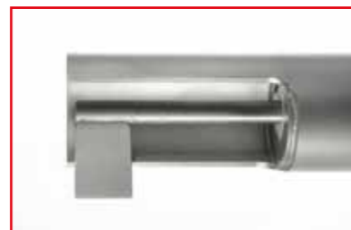
Paddle and shaft welded
