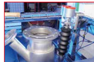
With bellows in a filling station for powdery, hazardous goods
