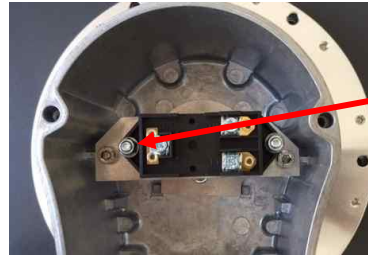
Avoid cavities forming in the adaptor!
